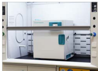
Removes fume from the inside of the chamber
