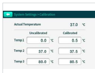
Accurate temperature control with 3-point calibration
