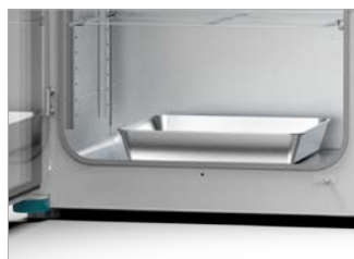
Water tray that minimizes media drying (option)
